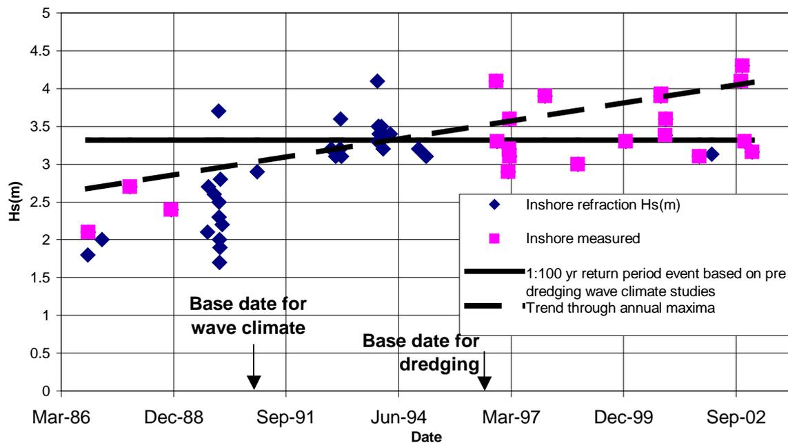
Figure 5 Temporal distribution of nearshore storm events resulting from storms with an offshore significant wave height >5m 1986-2003
