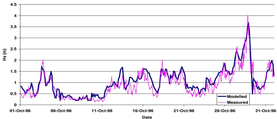
Figure 3 Comparison between modelled and measured wave heights at Milford-on-sea Waverider site
