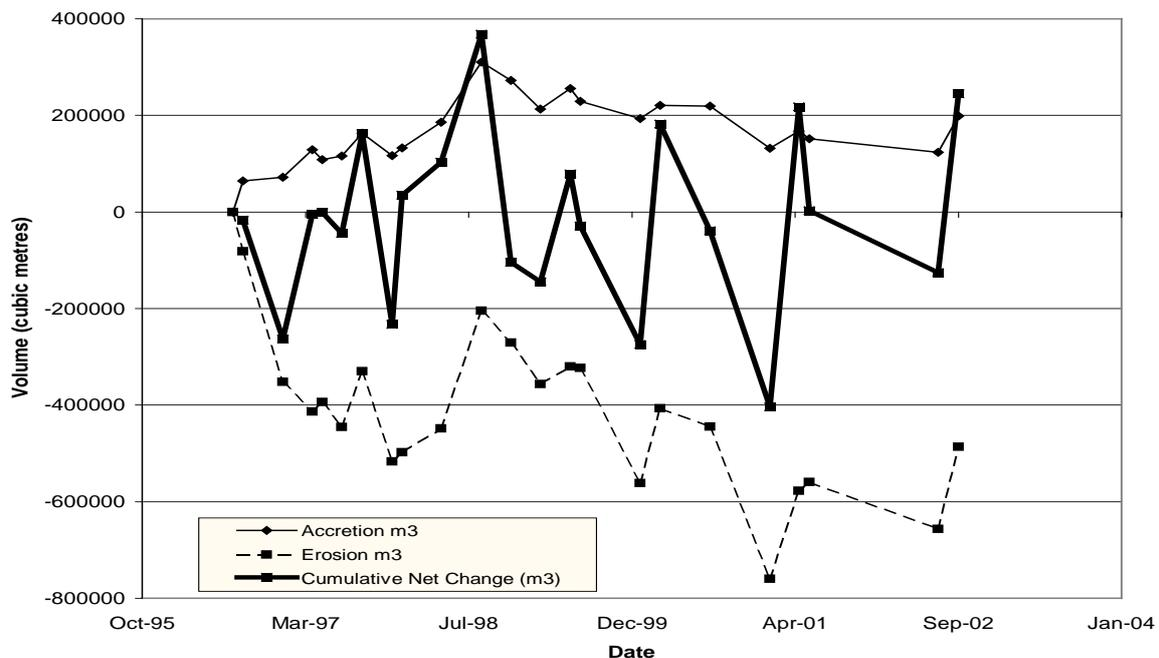
Figure 12 Volumetric Changes for Shingles Banks Dredging Area 406
