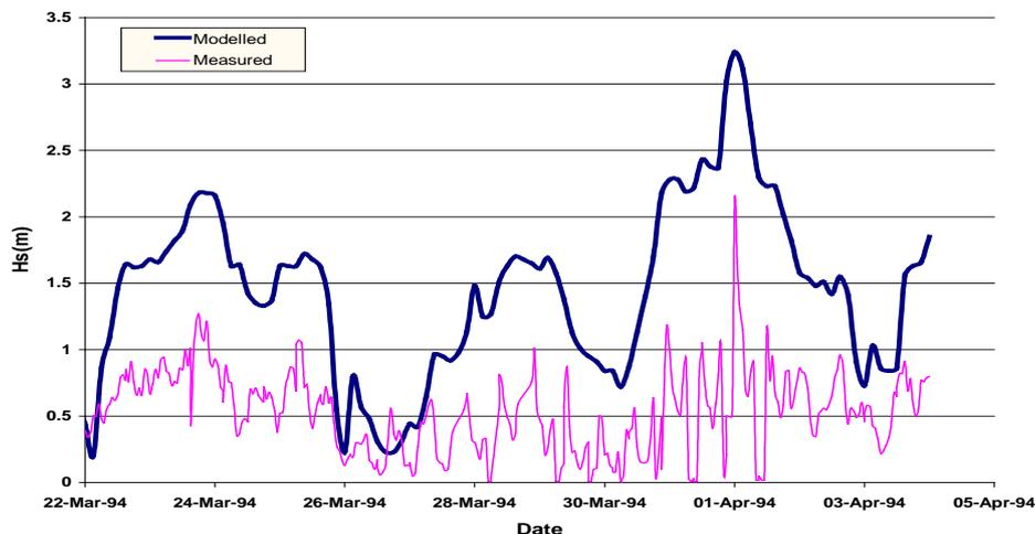
Figure 6 Comparison between modelled and measured wave heights at North Channel Waverider site
