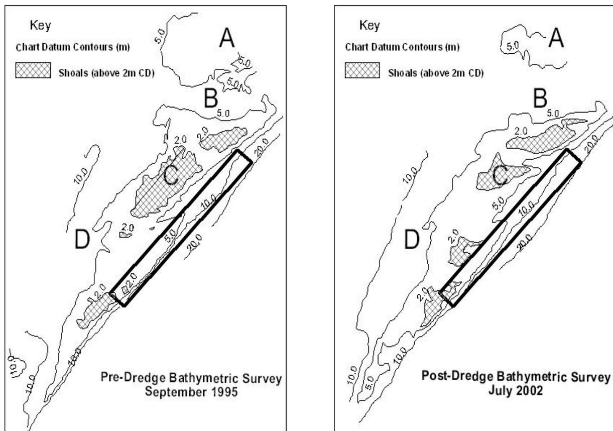
Figure 11 Evolution of the Shingles Banks system following aggregate dredging
