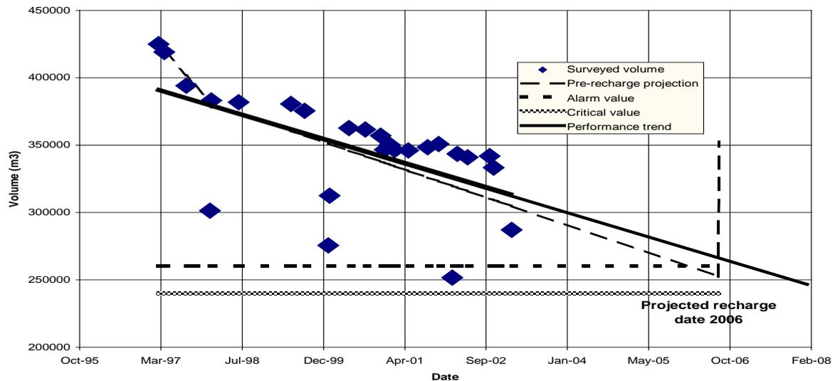
Figure 8 Comparison of surveyed and projected post recharge volumetric changes at Hurst Spit (above 0mODN)
