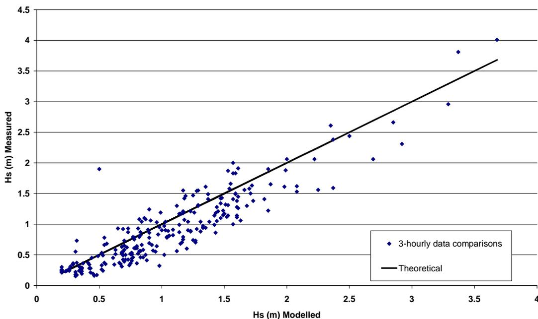
Figure 4 Correlation between modelled and measured wave heights at Milford-on-sea Waverider site
