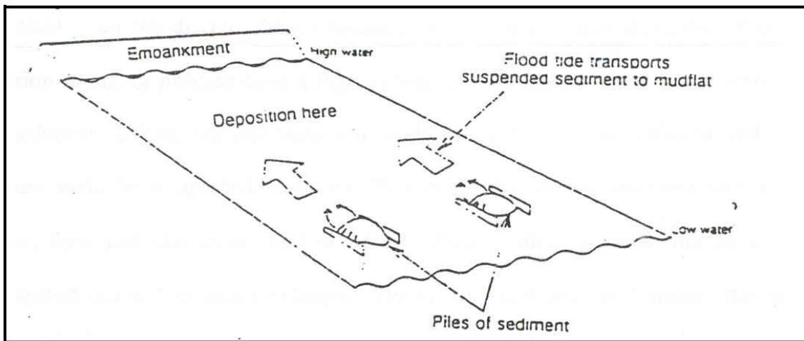
**Figure 2. Foreshore Recharge with Cohesive Sediments : Trickle Charging. Source: MAFF (1993).**
