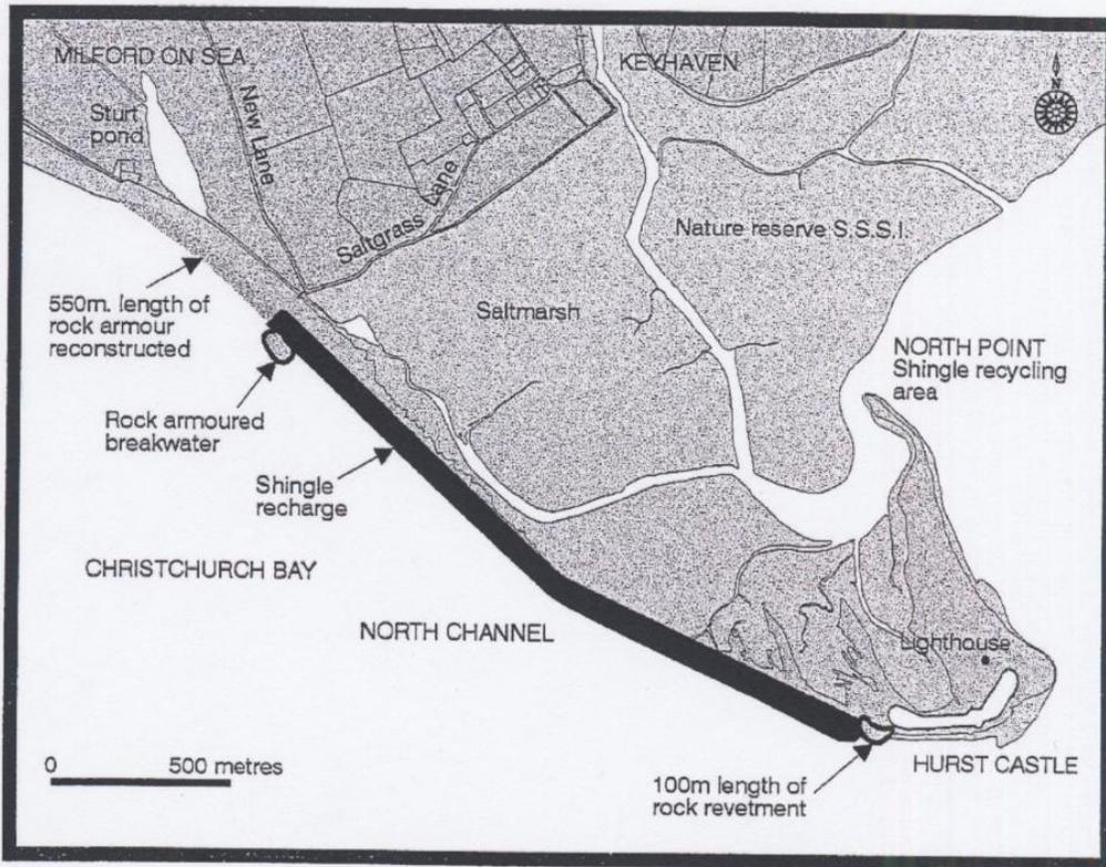
Figure 3 Plan layout of coast protection works at Hurst Spit
