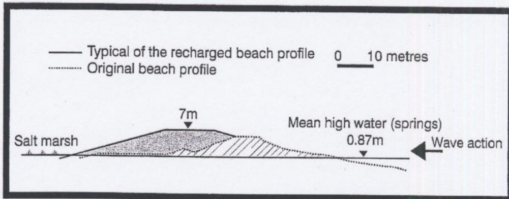
Figure 4 Typical cross section through beach recharge at Hurst Spit
